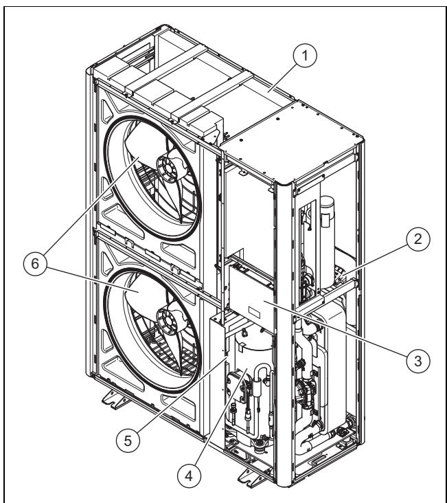
1 Evaporator                  2 INSTALLER BOARD PCB
