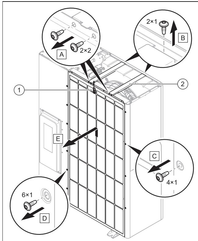
1. Disconnect the electrical connection to the temperature sensor (1).
