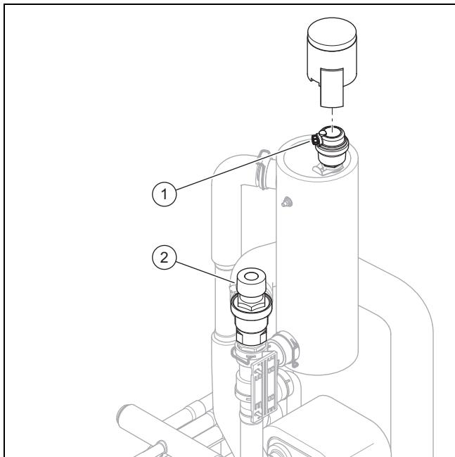
1. Remove the cap from the automatic air vent (1).
